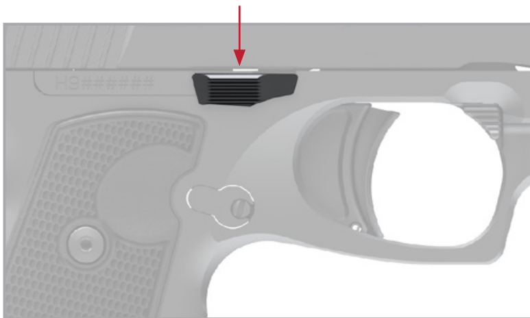
Figure 10: Slide Stop Lever Operation
