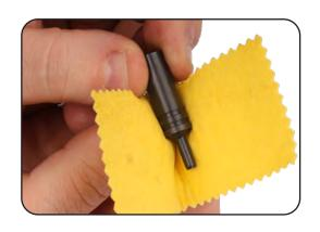
e. Clean the parts of the firing pin (firing pin, firing pin spring and locking pin).
