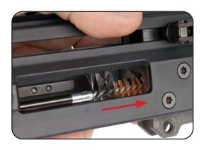
c. Using a small brush, clean the locking lugs on the bolt head, the bolt face and all guiding surfaces of the cam pin, bolt head and bolt carrier and then lubricate with a film of oil.
