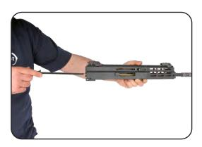
b. Clean the chamber with a short cleaning rod and a large brush.
