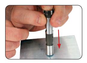
I. Use a punch to push the locking bolt out of the bolt head.
