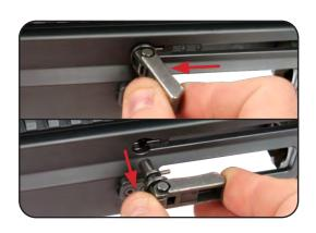
b. Pull both charging handles sideways out of the receiver.
