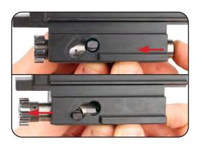
o. Insert the Bolt into the upper Receiver..
