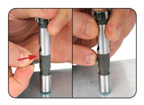
j. Insert the bolt head into the bolt carrier from the front.
